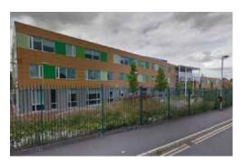
We used SGA's AA541 top hung windows along with anodised window pod flashings installed in to preformed apertures to give the building a truly distinctive appearance
